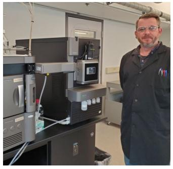
Chemist Andrew Barker works on the Laboratory's new LC-MS/MS to test drinking water for PFAS contaminants.
