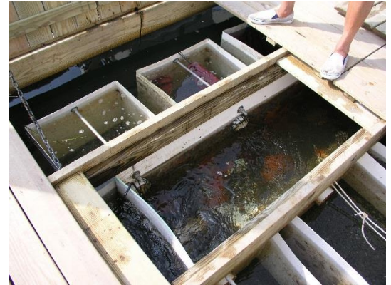
Figure 2 A FLUPSY or Floating Upweller System
