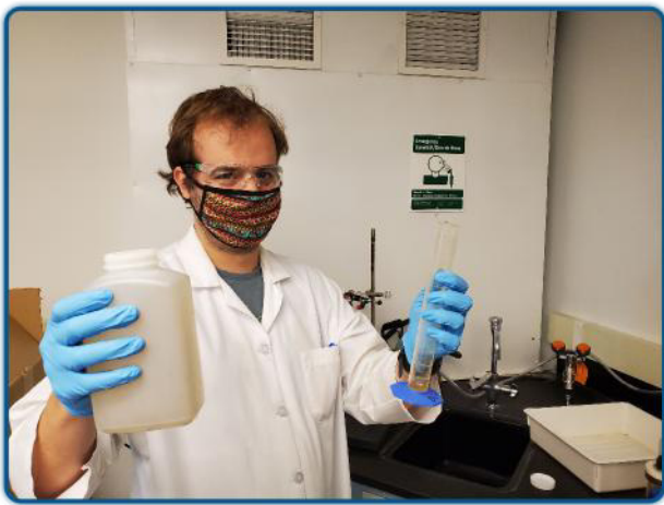
Chemist Steve Lee performing Total Suspended Solids analysis on wastewater samples from the Massachusetts Alternative Septic System Test Center.
