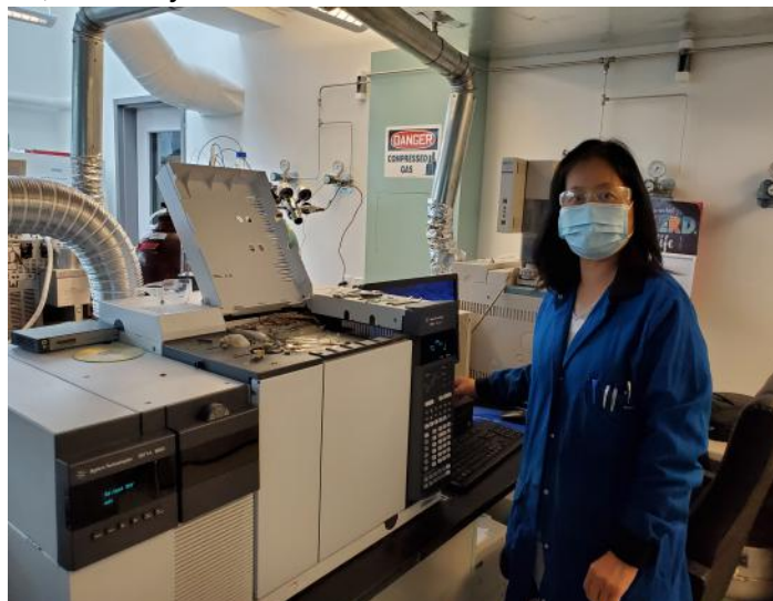
Chemist Liping Xun Analyzes a Sample for Organic Compounds using a Gas Chromatograph/Mass Spectrophotometer
