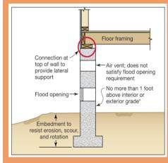
Flood vents installed in the crawl space allows water to pass through freely, reducing the water pressure on the building's foundation.
