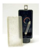
There can also be mercury in the hood and trunk light tilt switches of automobiles—as well as antilock brake systems, high intensity discharge (HID) lamps and automotive security systems.
