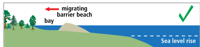
System migrates landward across the shelf as sea level rises.
