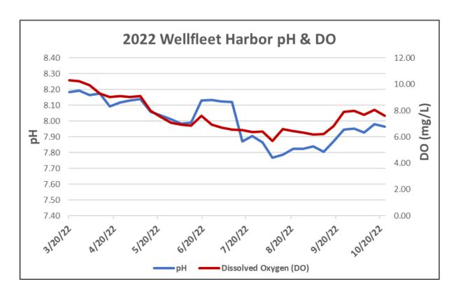
Weekly mean pH and dissolved oxygen as measured in Wellfleet Harbor during 2022.
