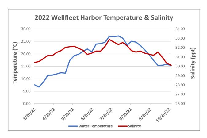
Weekly mean water temperature and salinity as measured in Wellfleet Harbor during 2022.
