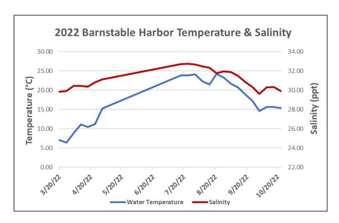
Weekly mean water temperature and salinity as measured at Scudders Landing in Barnstable Harbor during 2022.
